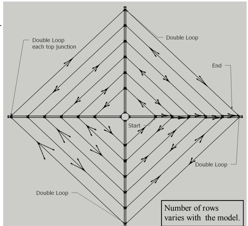
**NOTE: Some ropes are continuous and some are sectioned to avoid curling of rope during installation.**
